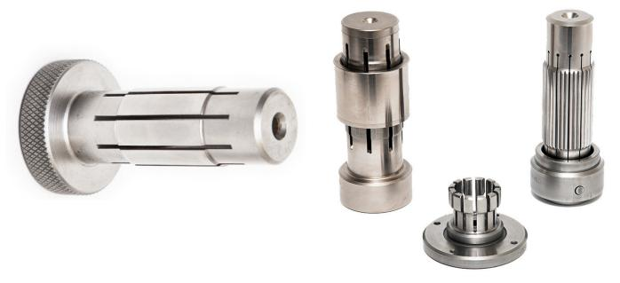
Built of one-piece construction, ground between centers, and no moving parts proved to be an extremely accurate yet inexpensive inspection arbor. Conforming to the part is excellent for checking the ID to OD, parallelism of the part faces, and perpendicularity.
