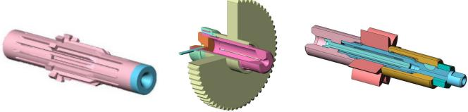
Using this same technology, arbors and chucks have been designed to grip not only in the ID but also on the OD, between centers, or flange mount. They are used to centralize with clamping devices, for part transfer, and more.
